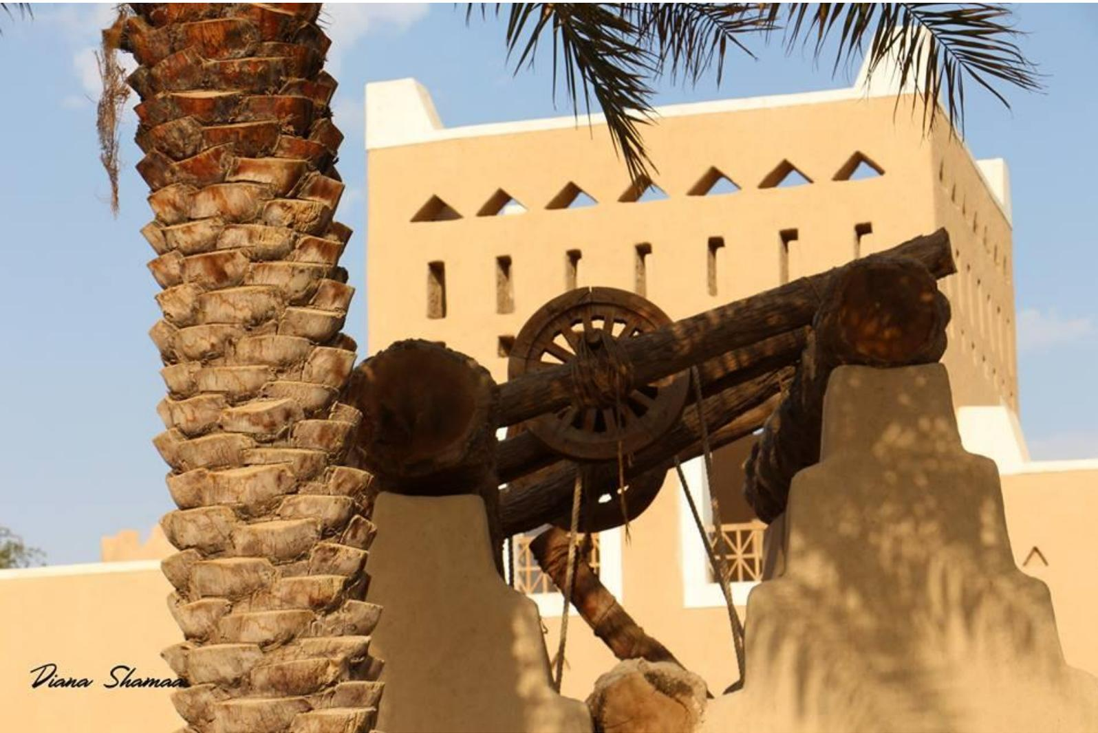
The *Sawani* is a contraption that was used in the past for extracting water which was used for drinking and for irrigations. The wooden wheels that were positioned above the well, four camels would usually make the wheels spin, as they spin water would be extracted from the underground. This is one of the few examples of ingenious vernacular technology.
